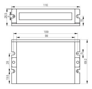
Figure 1: Mechanical specifications
