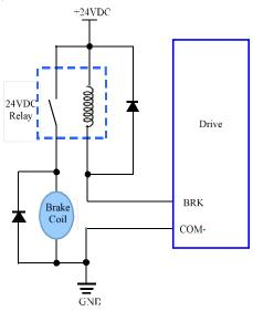
Figure 9 Brake output connection
