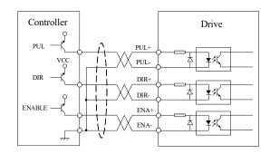
Figure 6: Connections to PNP (common-cathode)
