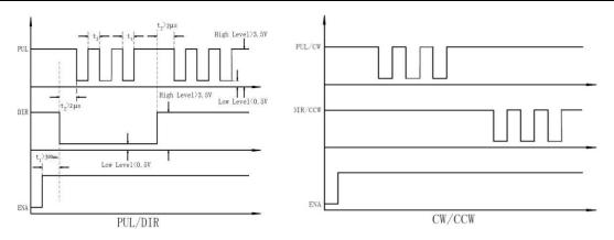
Figure 10: Sequence chart of control signals
