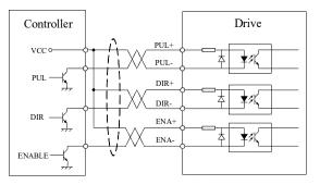
Figure 5: Connections to open-collector signal signal (common-anode)
